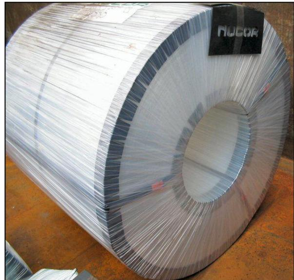
The Coilmaster MK 1 is the simplest version where the coil is delivered to the machine by crane or forklift for wrapping. As well as standard stretch and VCI films, strength films can also be applied to the coil. Edge-protection made from plastic or paper can be applied to the coil outer edge and bore during the main wrapping operations.
