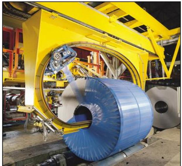
The powered film shuttle can apply a range of corrosion inhibiting films to the coils as well as protective films, strength films and also woven wrapping if needed. Depending on the options selected the machine is also able to apply coil outer edge plastic edge-protection automatically during the wrapping process. A highly flexible packaging systems solution from Signode.
